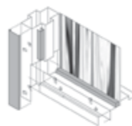
SILL / MULLION DETAIL WITH GLASS STOP
